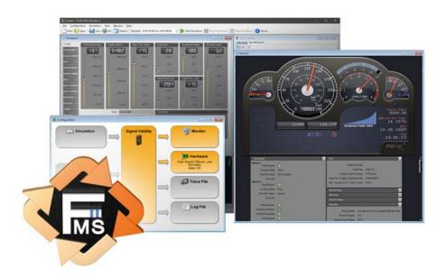
Windows Software for Simulating CAN Data According to the FMS Standard
